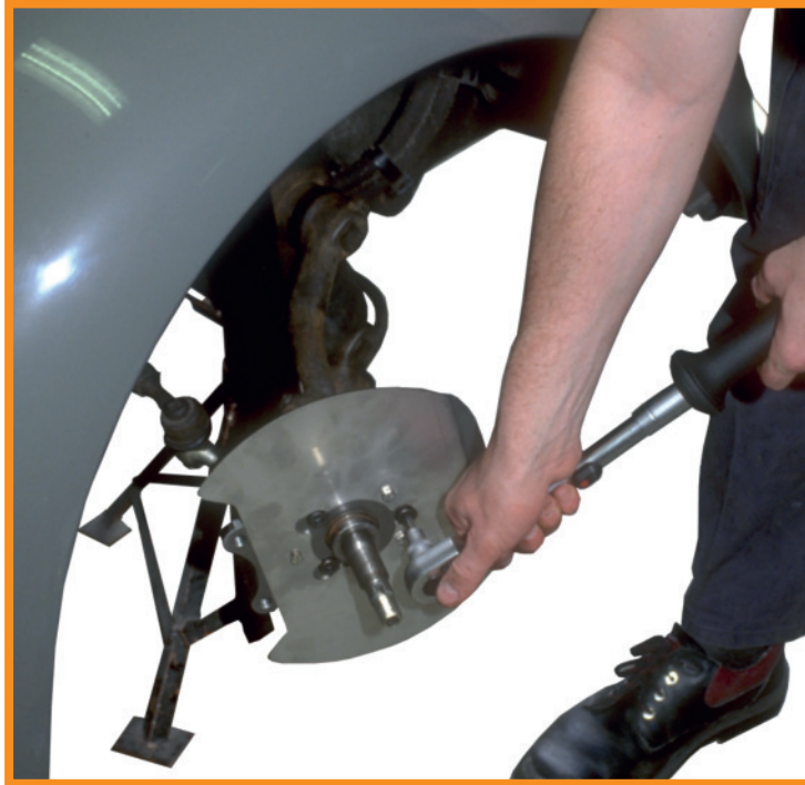
Fig. 5 Staubschutzblech Montage/ mounting the dust covers
