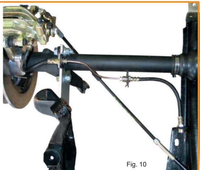
**CAUTION:** Be sure to route the hose in a smooth curve and check that it is not twisted. Also make sure that the hoses do not get in contact with any rotating or chassis parts.
