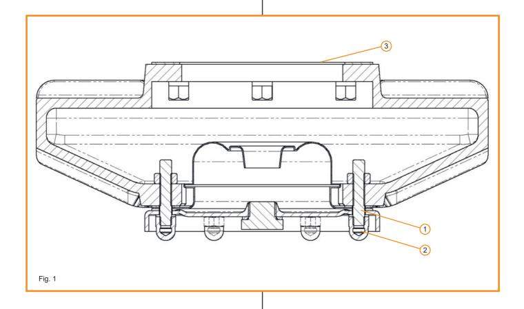
NOTE: The screw-in depth of the stud bolts is very important for the tightness of the cap nuts. If the thread of the stud bolt is too long, the cap nut cannot be screwed on far enough and therefore does not seal.
