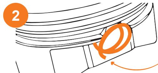
*The lock can then be spiraled into position as if you were screwing it into a groove (Fig. 2). After installation, it should no longer be possible to turn the lock by hand. Our CSP pistons require two Spiro Locks per piston, located at each end of the pin.*
