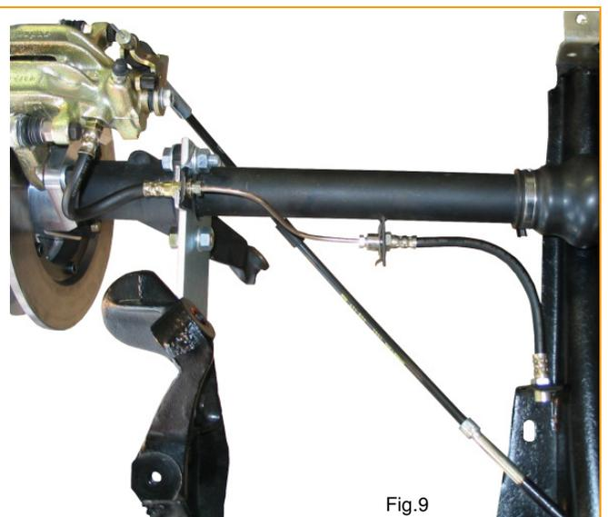
the handbrake lever (inside the car) into the chassis tubes, until the cable protrudes through the tubes which exit on the side of the rear frame forks.
